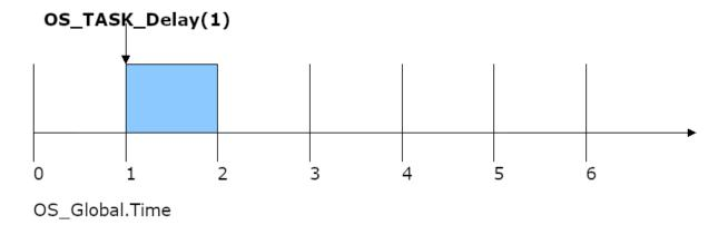
But if OS\_TASK\_Delay(1) is called shortly before the next timer interrupt the actual timeout will be less than a full system tick or even almost zero.
