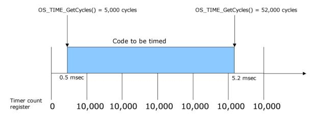
The first call to  $OS_{TIME\_Get\_Cycles()}$  returns the starting value at 5,000 cycles, while the second call to  $OS_{TIME\_Get\_Cycles()}$  returns the ending value at 52,000 cycles. The measured execution time of the code in this example would therefore be (52,000 cycles - 5,000 cycles) = 47,000 cycles, which exactly equals 4.7 millisecond.
