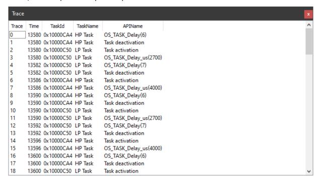
Every entry in the **Trace list** is recorded with the actual system time. In case of calls or events from tasks, the task ID (**TaskId**) and task name (**TaskName**) (limited to 15 characters) are also recorded. Parameters of API calls are recorded if possible, and are shown as part of the **APIName** column. In the example above, this can be seen with OS\_TASK\_Delay(6). Once the trace buffer is full, trace is automatically stopped. The **Trace list** and buffer can be cleared from embOSView.
