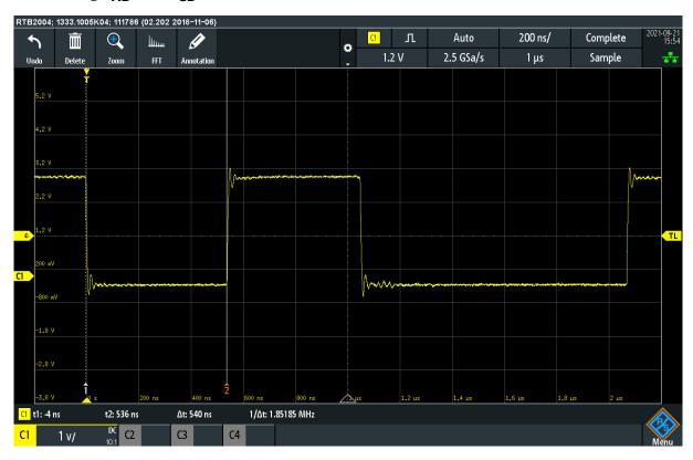
$t_{AB}$  is measured as 540ns.
