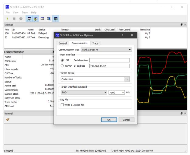
In the Communication tab, choose "J-Link Cortex-M (memory access)", "J-Link RX (memory access)" or "J-Link ARM7/9/11 (DCC)" in the  ${\tt Type}$  selection list box.
