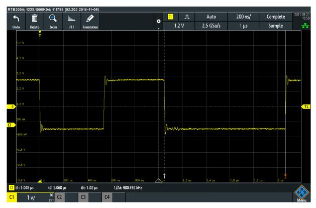
$t_{\text{CD}}$  is measured as 1020ns.
