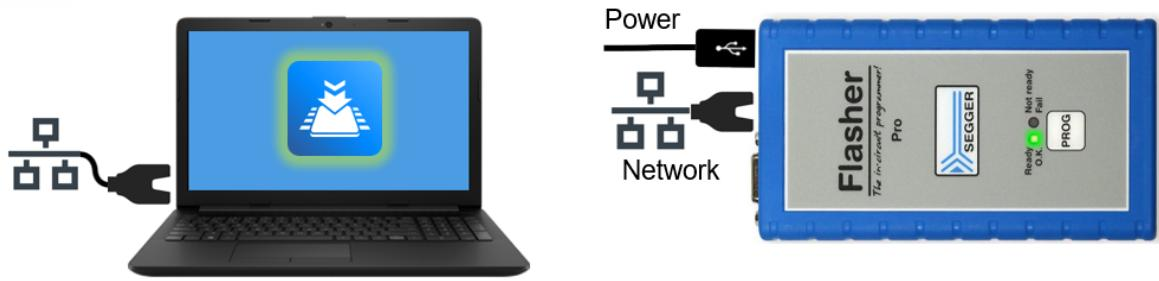
The Flasher Pro will obtain an IP address via DHCP, after which the green Ready / OK LED will slightly flicker once a second. You can check the IP address assigned to the Flasher Pro using the Flasher Configurator utility (also see further below).
