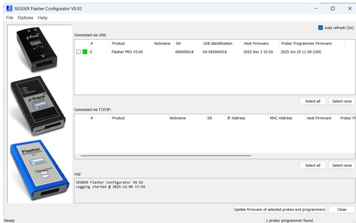
If Flasher Configurator detects that a firmware update is available for the Flasher, it will indicate this by marking the programmer firmware version as "Old" (as shown in the screenshot above).
