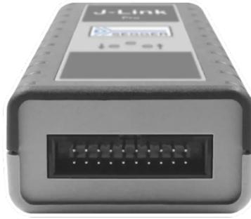
The pinout for the 20-pin, 0.1"-pitch debug connector depends on the debug interface used.
