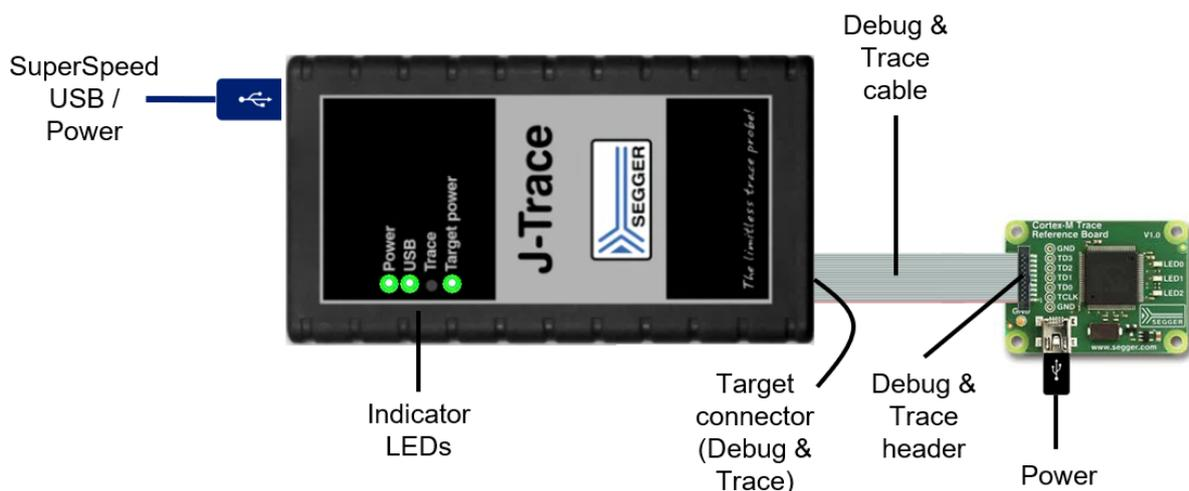
J-Trace ships with a 20-pin, 0.05"-pitch ribbon cable. In rare cases, depending on the target board, you might need a separate trace adapter.
