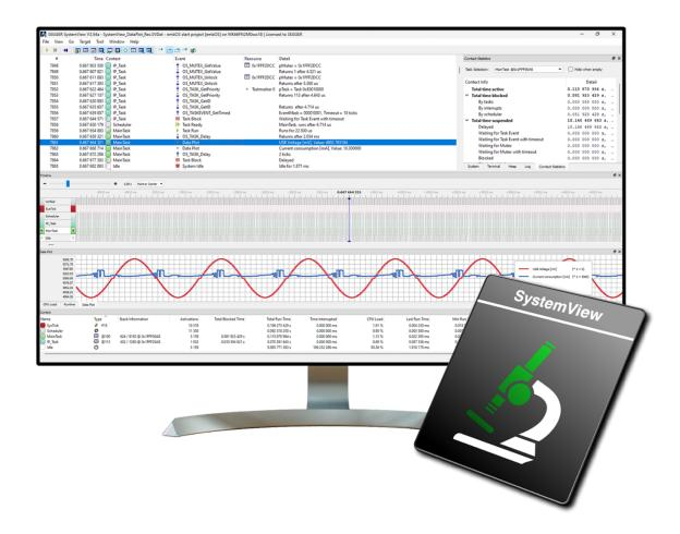
SystemView provides powerful features while being minimally intrusive, which makes it an essential tool for embedded system development. It works with any CPU, RTOS, or baremetal system, ensuring high flexibility and adaptability to different setups. With this broad compatibility, developers can use SystemView in a wide variety of embedded projects.
