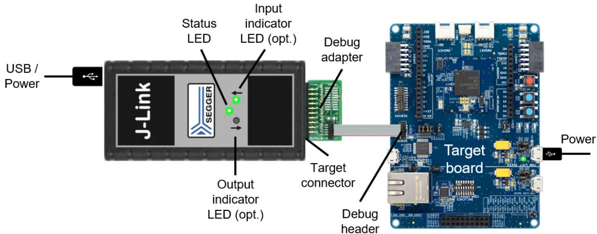
Connect the debug adapter (or the 20-pin ribbon cable, if possible) to the J-Link target connector as well as the debug header on the target board as shown in the image above. Watch out for the correct orientation. The colored wire of the ribbon cable needs to connect to pin 1 of the debug header. Also make sure the connector covers both rows of the debug header.
