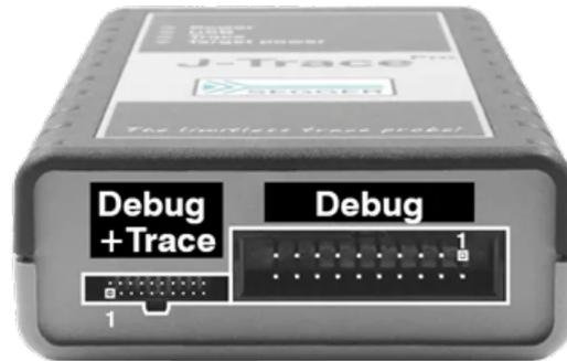
The 20-pin, 0.05"-pitch debug & trace target connector is used for advanced debugging (instruction trace, code coverage, code profiling, etc.). The pinout of this connector can be found in the SEGGER knowledge base:
