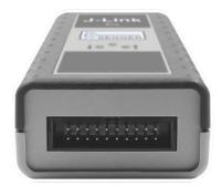
The pinout for the 20-pin, 0.1"-pitch debug connector depends on the debug interface used.
