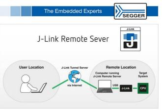
effective use of scarce hardware. Cloud-based development systems can debug a target system on the developer's desk. The same applies to SEGGER flash programmers. Flashers in use far away can be controlled, monitored and updated.
