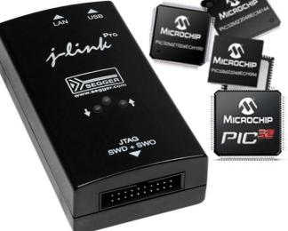
not different when it comes to debugging PIC32 devices. In addition, the J-Link allows setting an unlimited number of breakpoints in flash memory.
